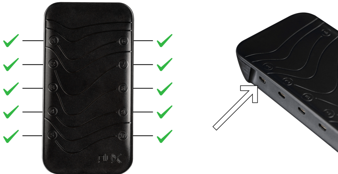
Figure 2: Compatible Biosignals PRO ports and example of Port 1.
