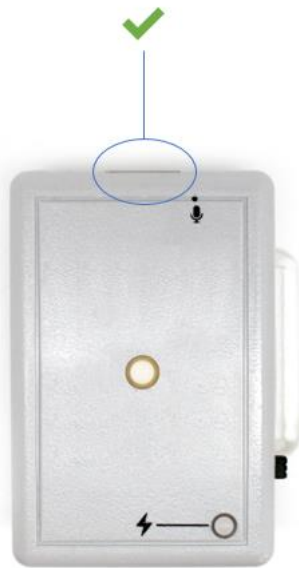
Figure 8: Connect the ECG to the analog input channel of the biosignalsplux Solo (openBAN).
