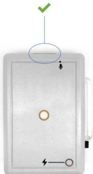
Figure 7: Connect the BVP to the analog input channel of the biosignalsplux Solo (openBAN).
