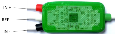
Fig. 2. Assembled EGG sensor – inside view with connection pins (IN+/- and REF).
