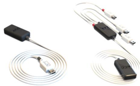
Fig. 1. Assembled ACC sensor – Z (left) and XYZ (right).
