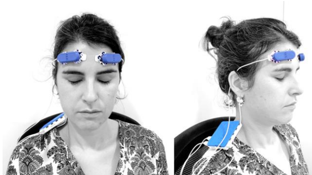
Fig. 4. Example of the sensor placement for 2-channel EEG acquisition on the forehead (Fp1 and Fp2 positions in the 10-20 EEG system placement); front view (left) and side view, including the placement of the reference cable (right).
