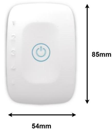
Fig. 1. 4-Channel biosignalsplux hub dimensions.
