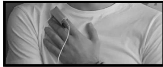
Fig. 3. Sensor Placement (forefinger)
