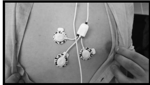
Fig. 3. Sensor Placement (V2 configuration)
